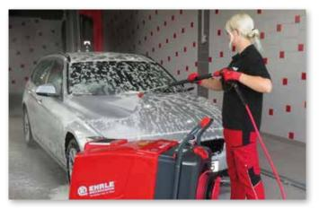
Car cleaning with lance and stainless steel flat jet nozzle
