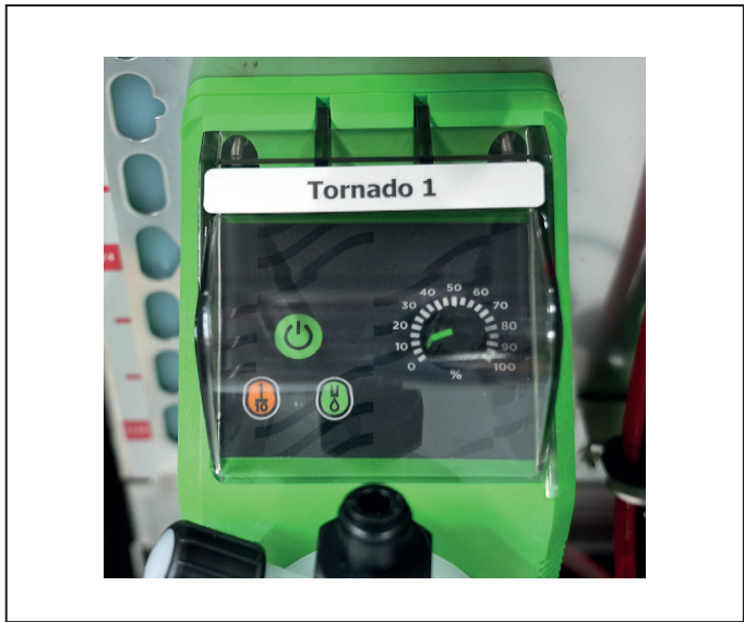
Fig. 4 - 9 Dosing controller for operating setting of Tornado Nozzle dosing pump
